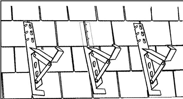
ROOF JACKS NAIL IN THE SLOT OVER STANDARD THICKNESS SLATES WITH 16P COMMON NAILS, AND UNDER THICK SLATES (AS SHOWN IN THE CENTER) TO HOLD A 2X10 PLANK. A LADDER CAN BE SET ON THE PLANK AND LAID ON THE ROOF. ALTERNATIVELY, REMOVE A SLATE AND NAIL THE ROOF JACK BETWEEN THE TWO UNDERLYING SLATES.
